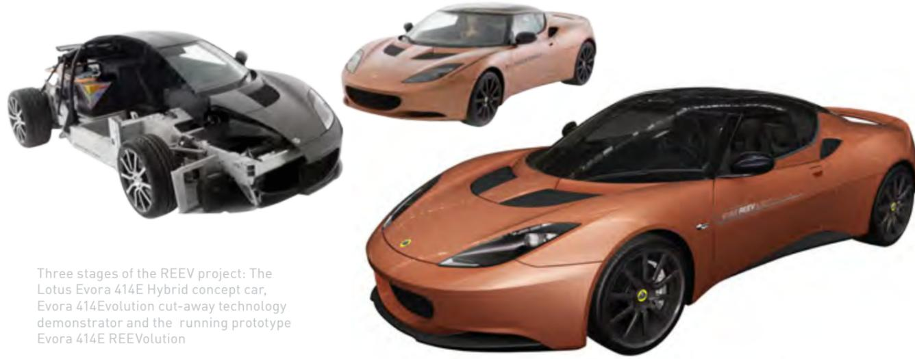
Three stages of the REEV project: The Lotus Evora 414E Hybrid concept car, Evora 414Evolution cut-away technology demonstrator and the running prototype Evora 414E REEvolution
