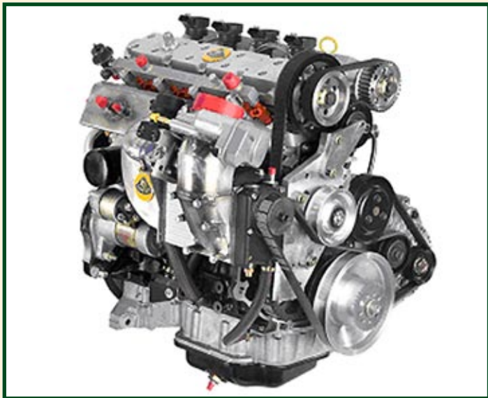
Lotus pressure charging concept engine
