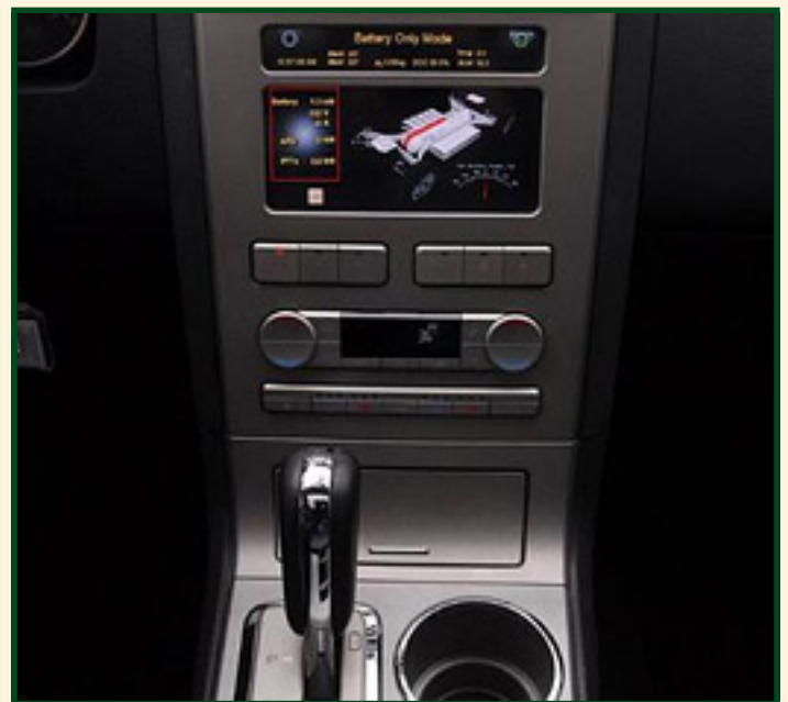
A screen helps the driver tell how much battery power is being drained, promoting efficient driving
