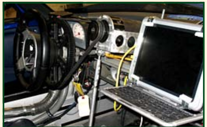
Belt and pulley drive for steering Lone Wolf
