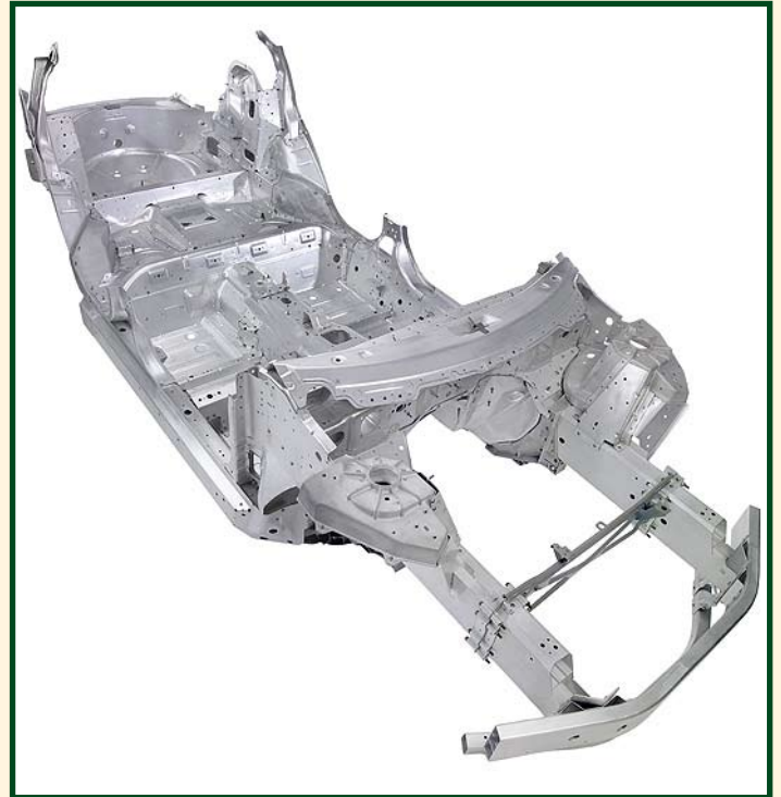
Lotus VVA – an example of a fully riv-bonded structure
