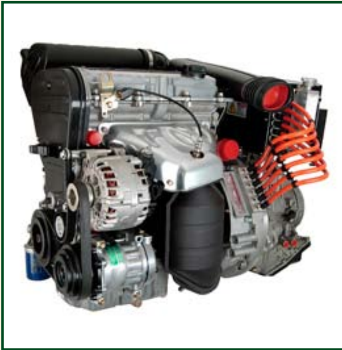
The base CamPro engine mated to the motor/generator and CVT
