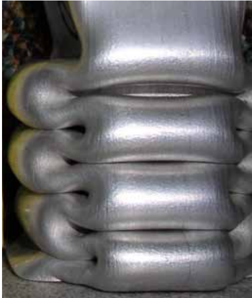
Ideal energy absorbing crush behaviour
