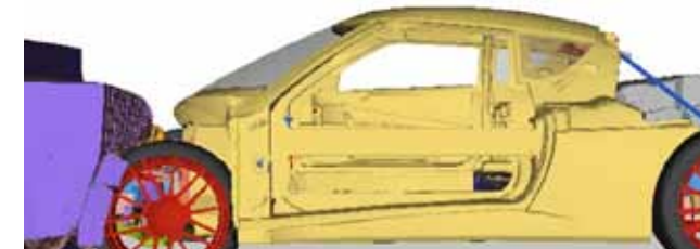
European legislative 35mph Offset Deformable Barrier (ODB) impact simulation and test
