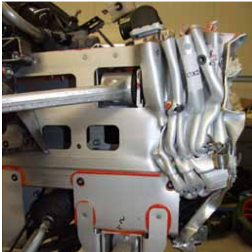
"Real World" energy absorbing crush behaviour
