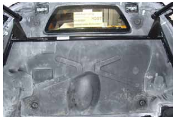
Rear bulkhead area after Federal legislative 50mph rear impact showing negligible deformation
