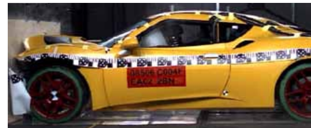
European legislative 35mph Offset Deformable Barrier (ODB) impact simulation and test
