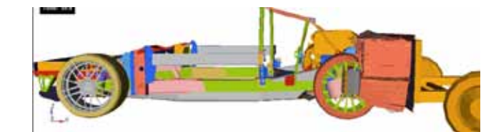
Federal legislative 50mph rear impact simulation and test
