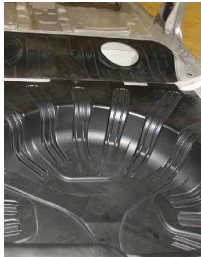
A glass-mat thermoplastic (GMT) wheel well
