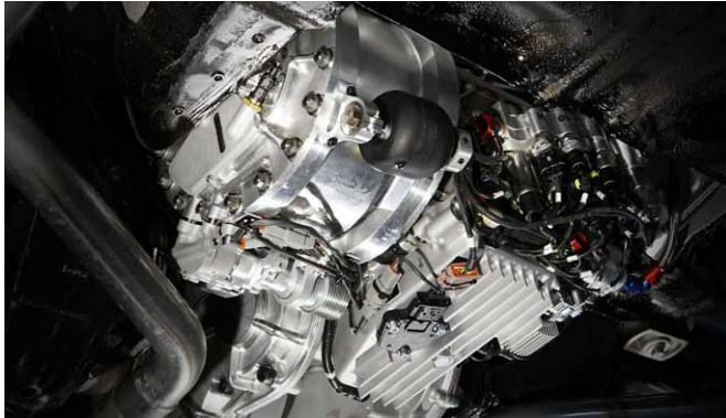
Flywheel CVT installation
