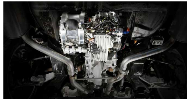
Flywheel CVT installation
