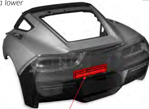
The new 2014 Chevrolet Corvette uses a lightweight heat-activated shape memory alloy wire in place of a heavier motorized part to open a vent that allows the trunk lid to close more easily.
